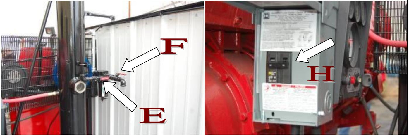
Before you engage Vacuum Pump increase engine RPM to 1400 RPM and then back down to 1000 RPM. This gives the alternator a chance to build voltage to support the pump and battery.
